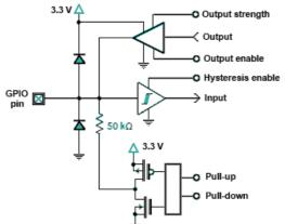
Fig. 5 Equivalent circuit for a Raspberry Pi GPIO pin.
