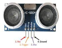
Fig 3 Ultrasonic Sensor
